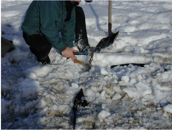
Locating edges of collection mat and lifting the mat off the frozen ground.
